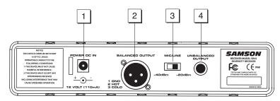
**1: DC input** - Connect the supplied 12 volt, 500 mA power adapter here, using the strain relief as shown in the illustration below. **WARNING:** The substitution of any other kind of power adapter can cause severe damage to the SR5 and will void your warranty.
